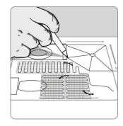
Plan the installation and mark where each run should go to ensure you have the correct size system. Now start to lay the Loose cable taking care not to cut or damage the cable with sharp tools. Wear soft-soled shoes throughout.
