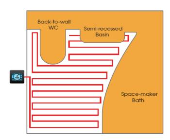
If necessary, you can adjust the spacing, although we recommend that you keep it as regular as possible. Any excess cable can be run around the perimeter of the room. Once installed we recommend another continuity/resistance check at this stage.
